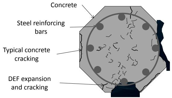
DEF is Delayed Ettringite Formation. Ettringite crystals form some number of years after the concrete is cast. They break up the concrete as they grow and significantly decrease the concrete's structural integrity.
